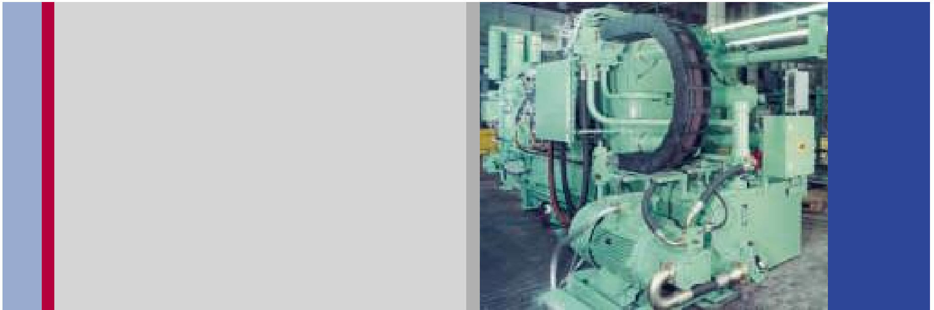
Pressure cast machine, pump with variable pump flow thanks to drive speed control
